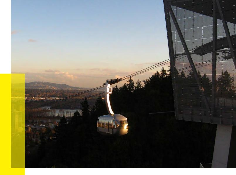
Cable Propelled Transit (CPT) is a family of technologies where automated, passive vehicles are propelled and often supported by industrial strength steel cables.
